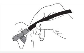
Cut off excess air line squarely. Install the air line into the fitting. Push the cut end of the air line into the selflocking fitting as far as it will go while slightly turning. A definite click can be heard and/or felt when the air line is seated. Air line should go in approximately <sup>9</sup>/<sub>16</sub>".
